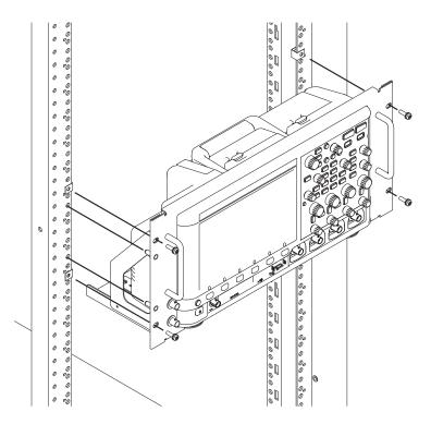
**3** Fasten the support shelf to the rack cabinet using four 10-32 dress screws. This completes the installation.
