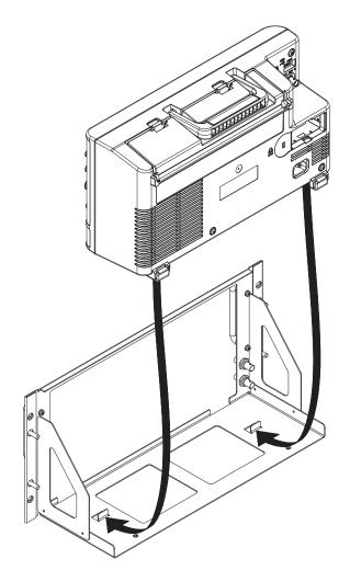
**2** Push the oscilloscope fully forward on the support shelf assembly.
